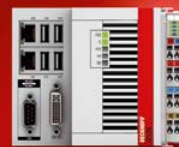
CX5120: Intel®-Atom™-CPU, 1,46 GHz, single-core
