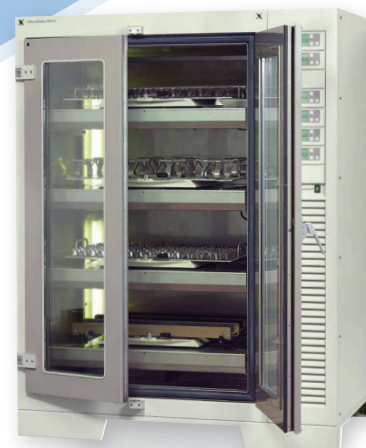
ISF4-X large incubator shaker with up to five independent height adjustable shaker units
